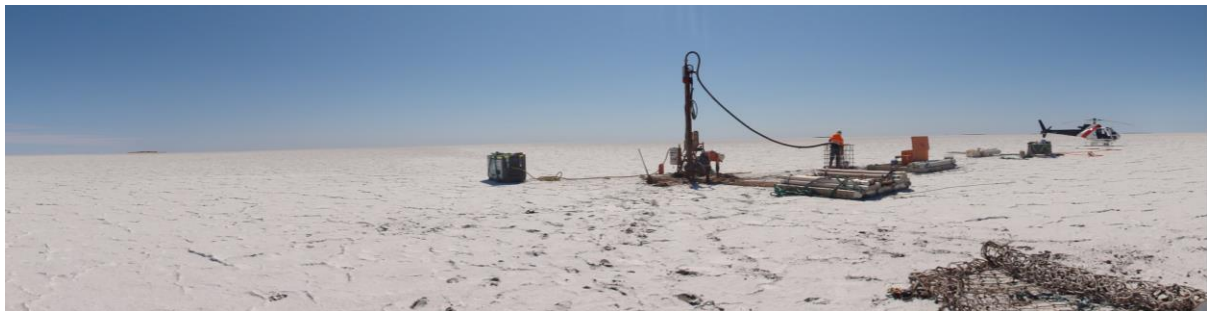
Figure 1. Aircore Drilling in Progress
