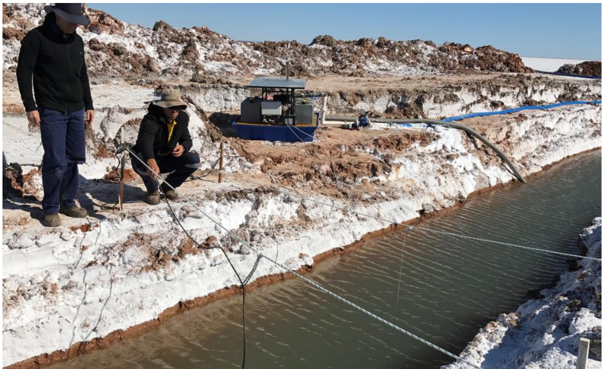
Figure 3. Pump Testing at Trench T3
